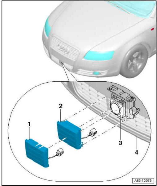
Removing and installing cover on vehicles with ACC (adaptive cruise control)
