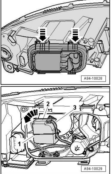
Note correct installation position: lug at top of bulb holder must engage in recess of gas discharge bulb.
