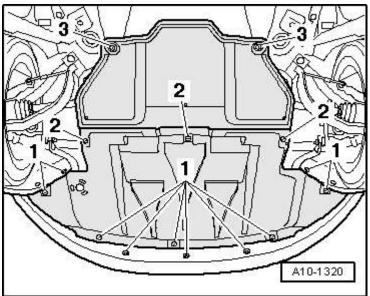
For this purpose, release bolts/quick-– release fasteners -1- and -2-. Leave quick-release fasteners -3- for noise insulation panel (rear) in position.
